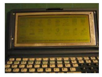
Now place the plastic bezel back to its original position and press down gently. The bezel would hold the polarizer in place.
