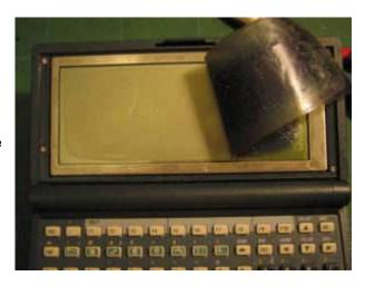
This is the one that's very tough to remove. If the damage hasn't "eaten" into this film, there is not need to remove this to save your time.
