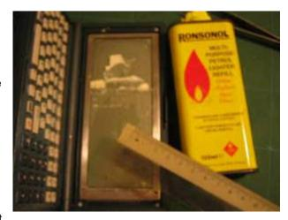
too much of the lighter fluid goes to the edge and do not remove the sticky bits around the bezel area. Lots of white powder like shavings would be formed but the lighter fluid will hold it all together.
